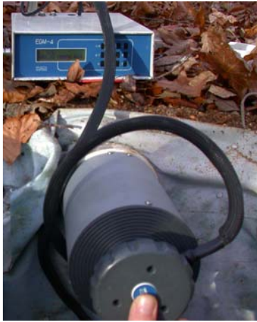
Figure 5. Picture of the EGM-4, which is used to measure SEF.
