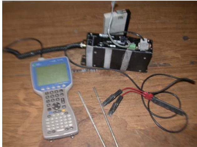
Figure 6. Picture of TDR 100, Allegro, and rods used to measure soil moisture.
