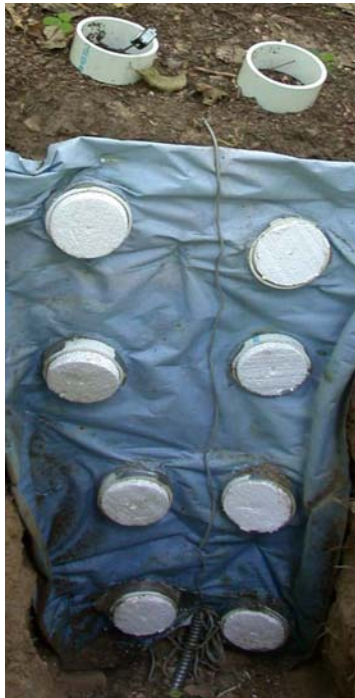
Figure 4. Installation of soil efflux measurements.
